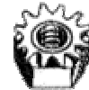
Kep A nut with a built in external tooth lock washer, used to speed up assembly.
