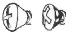
Oval A countersunk head with a rounded top. Abbreviated OH or OV
